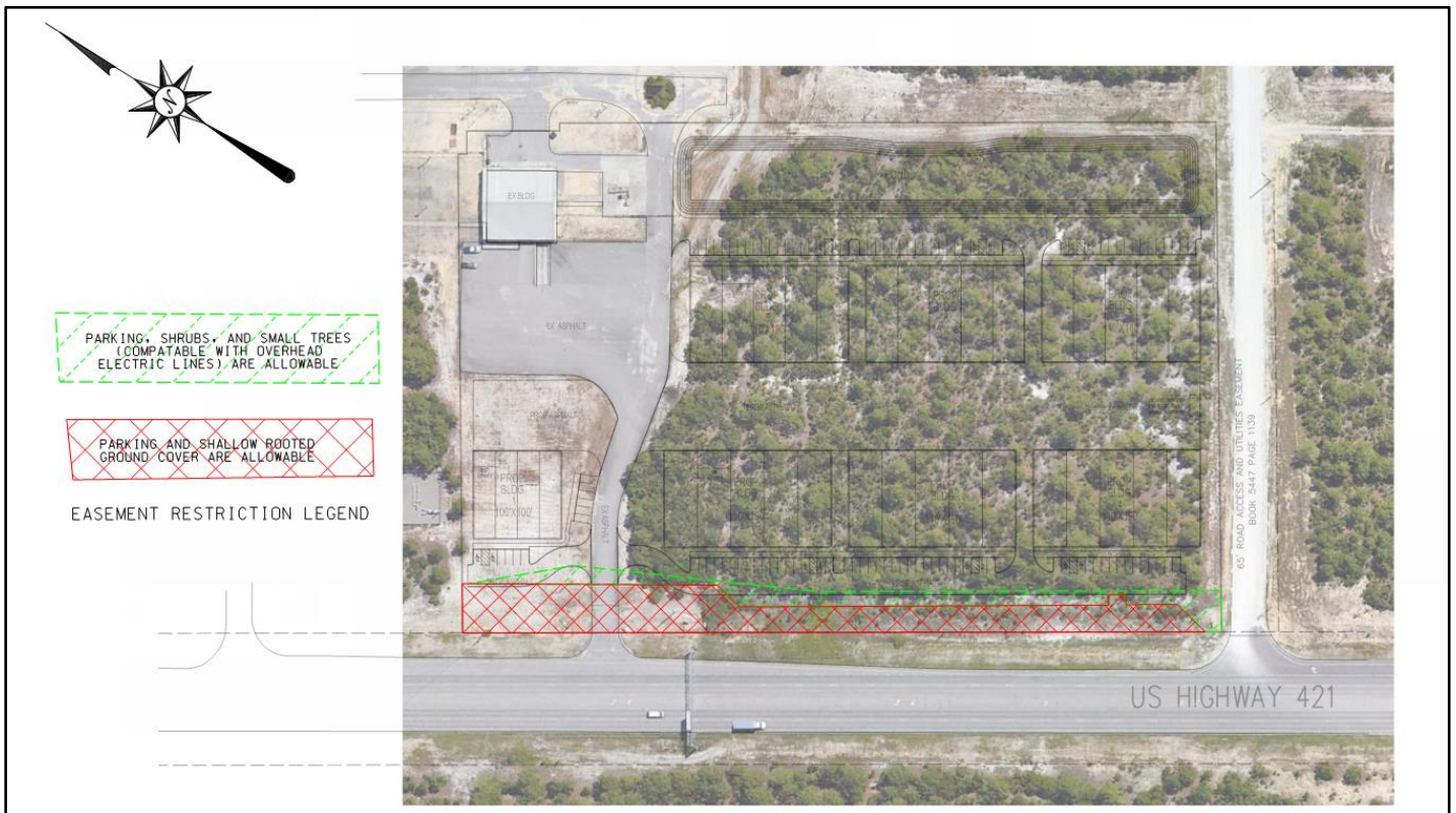
Figure 1: Recorded easements on property adjacent to US Highway 421 N in area of required landscaping.
