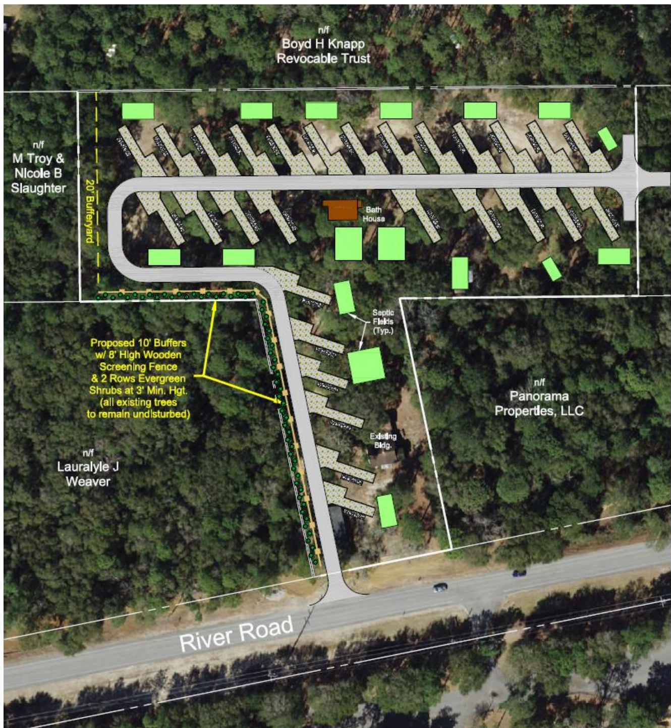
Figure 2: Conceptual plan with area of proposed transitional buffer variance.
